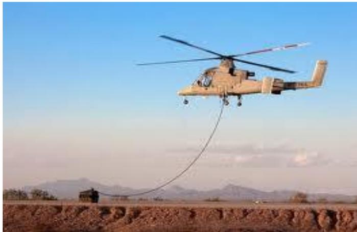
Fig.3. K-MAX unmanned helicopter conducting resupply operation<sup>12</sup>
