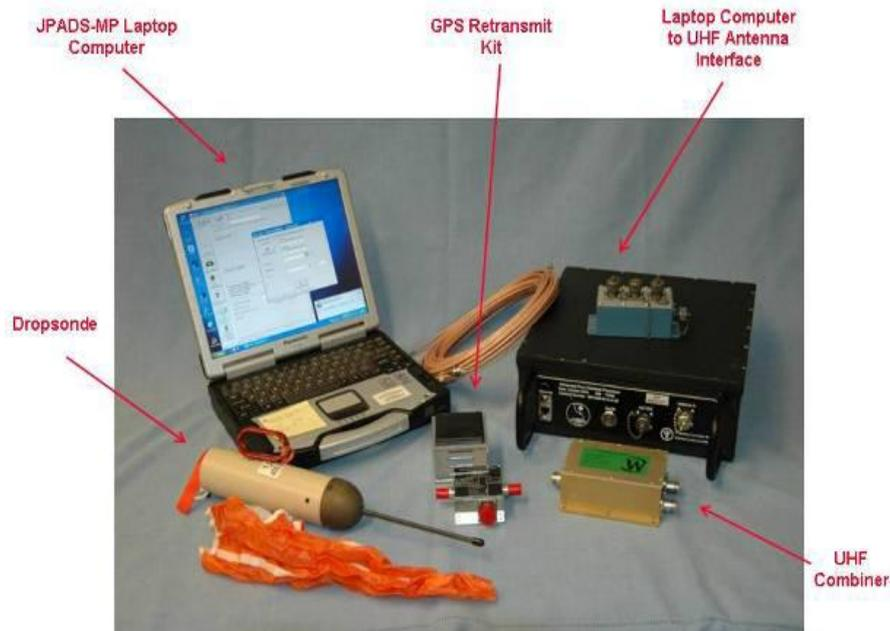
Fig. 7. USAF JPADS-MP primary components and carrying case<sup>19</sup>
