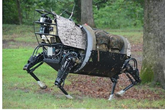
**Fig. 3. LS3 prototype**
