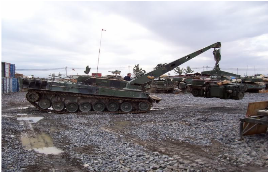
Fig. 6. Leopard 1 based ARV lifting a 4.7t Leopard 1 powerpack with full extended crane arm and without using any anchors also being able to transport it from a place to another 10 .
