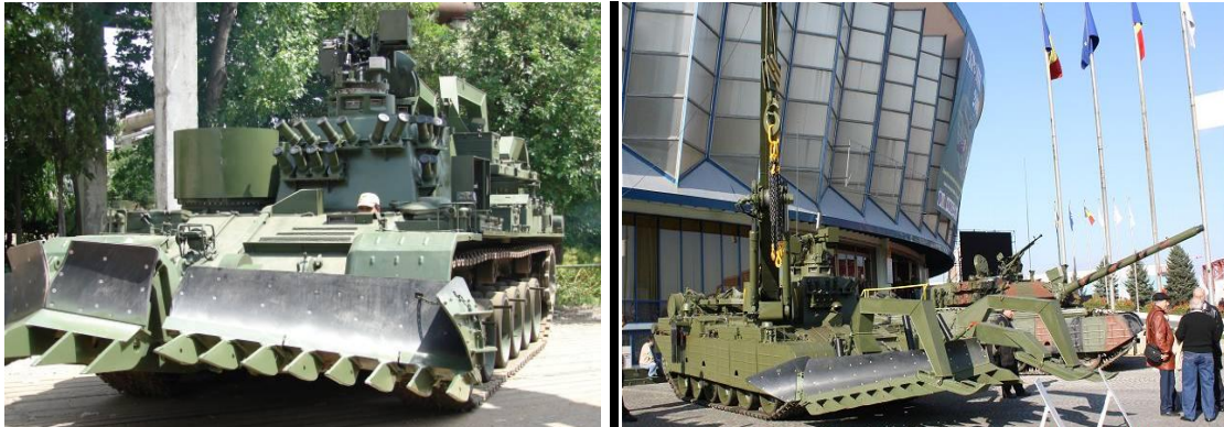
Fig. 7. Romanian DMT 85 a multi-purpose vehicle based on TR 85 tank chassis 11
