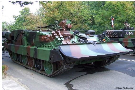
Fig. 5. Polish WZT 3 built on T 72 APC 77 chassis 7
